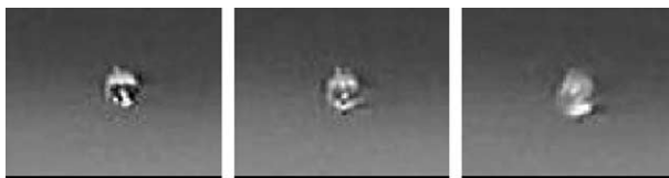
Fig. 2. A freezing droplet: not frozen drop (left), freezing drop (middle), frozen drop (right).
